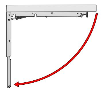
**7.** Lift the table top/shelf and test the function by pulling the release levers. If you use a Regal Soft, make sure the table top/shelf folds slowly.
