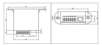
Fit the touch pad iat a location that is within suitable reach to allow for ease of operation. Make sure that sufficient room - at least 100 mm space available under the front of the touch pad - is available for the cables and the connectors. The required mounting hole for the touch pad is  $36.5 \times 21$  mm.
